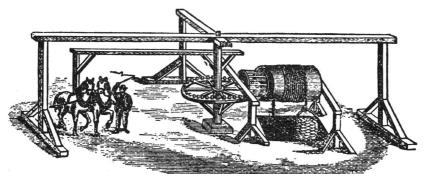
Figure 1. Horse Powered Winding Engine (From A Glossary of Scotch Mining Terms, Barrowman, J. 1886)
