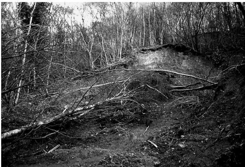
Figure 4. View from the toe of the main landslide in April 1999, showing the debris flow. Trees fell backwards (upslope) as their roots were carried down-slope. The toe of the main landslide intersected the channel of the Wharry Burn, but the height and volume of material was insufficient to cause a lake to form (photo April, 1999).
