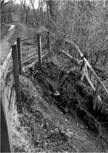
Figure 9. Detail from the middle slide in April, 2009. This shows widening of the slide as well as headward recession with renewed flows down-slope (net changes are probably around 0.5 m in each event).
