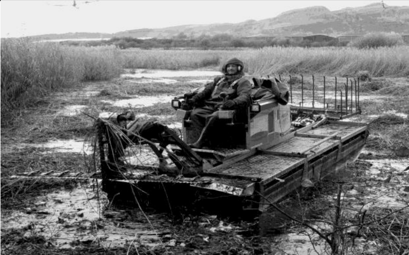
Figure 4. The Truxor amphibious reed cutter.
